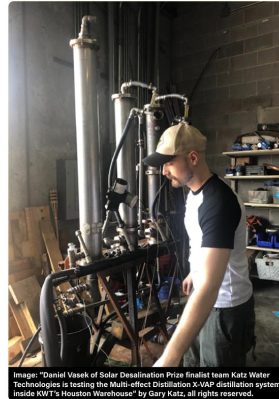
Image: "Daniel Vasek of Solar Desalination Prize finalist team Katz Water Technologies is testing the Multi-effect Distillation X-VAP distillation system inside KWT's Houston Warehouse" by Gary Katz, all rights reserved.
